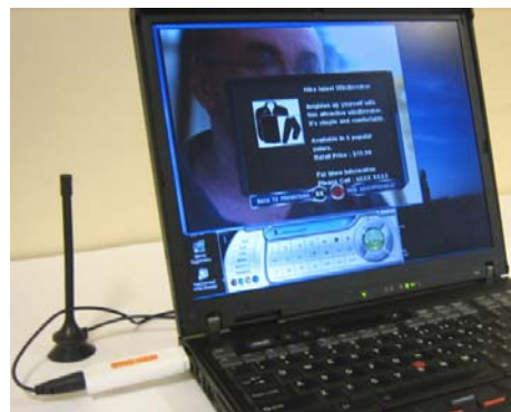
DVB-T USB Dongle and Mediastack-MHP
